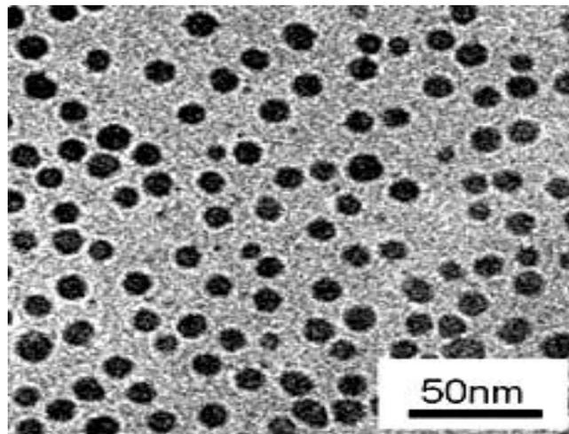
**Figure 6:** Scanning electron micrograph of silver nanoparticles
